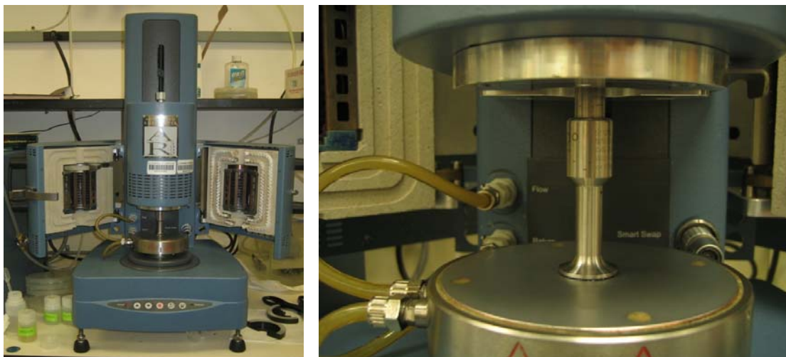
Figure 2.10: a) AR 2000 Rheometer, b) Cone-Plate Configuration
