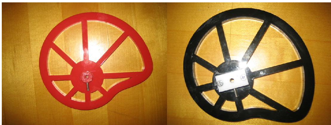
Figure 3.3: a) Initial low frequency cam, b) High frequency cam
