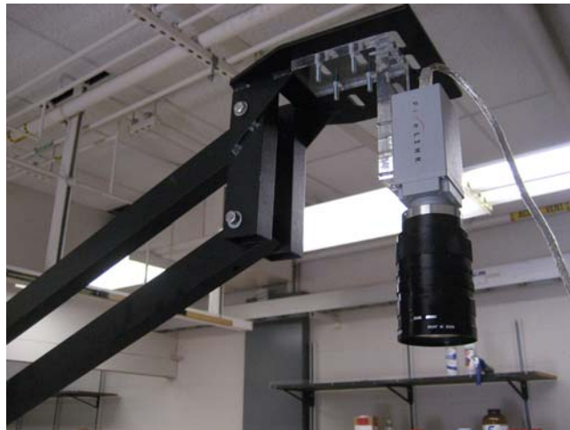
Figure 2.16: High speed camera on positioning boom arm
